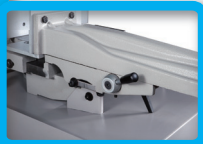
Push the handle, fast moving to open the vise
