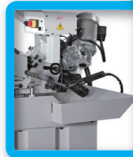
Moveable chips tank, easy to clean
