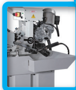
Moveable chips tank, easy to clean
