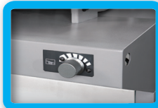
Feed down speed control
