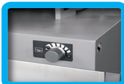
Feed down speed control
