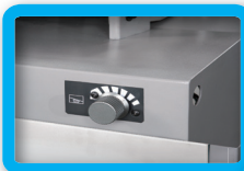
Blade Guide With Hard Metal Pad
