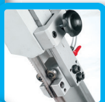
Blade Guide With Hard Metal Pad
